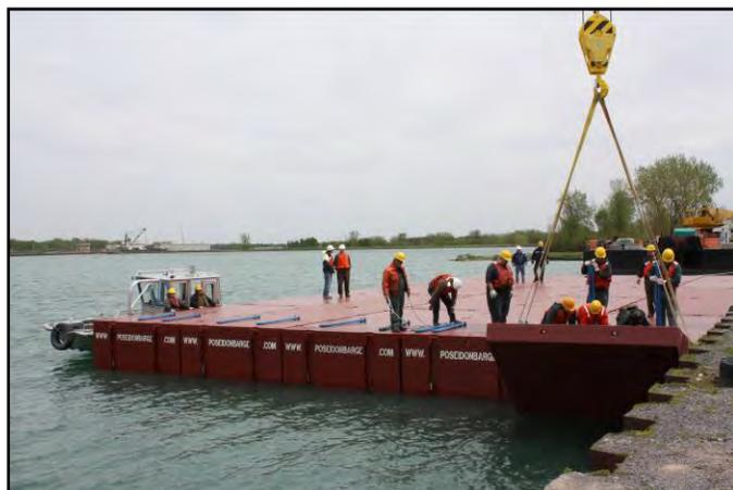
*Corporation personnel under the direction of Poseidon representatives are assembling the sectional spud barge for the first time.*
