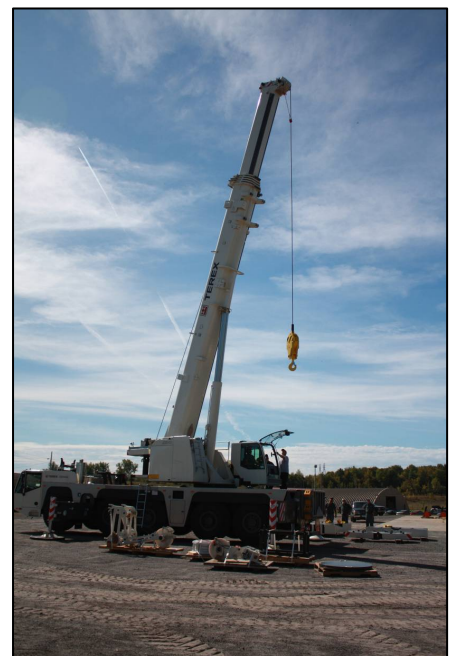
SLSDC's new 170-ton capacity all terrain crane
