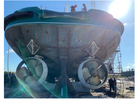
Lower Z-Drive units (size comparison to a person standing 5'9")
