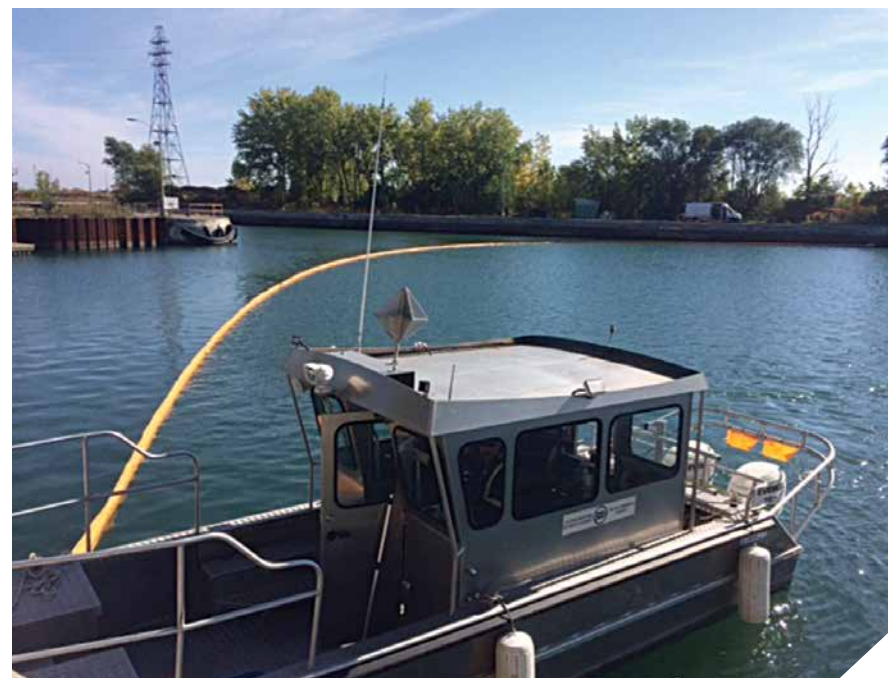
Containment boom being deployed at the Beauharnois Locks during a simulated oil spill in 2014.
