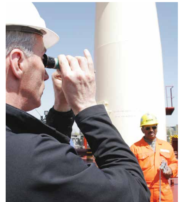
Seaway Inspector Robert Elliott verifying the salinity of a ballast water sample
