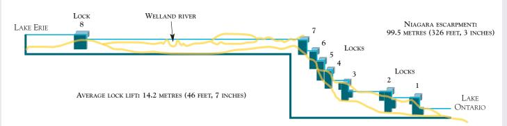
The seven lifts are located in the northern 11.6 km (7.2 miles) section of the canal, between Lake Ontario and the top of the Niagara escarpment. A 27.8 km (17.3 miles) man-made channel runs through level ground to the shallow-lift control lock at Lake Erie. Piers projecting into the lakes account for an additional 4 km (2.5 miles).
