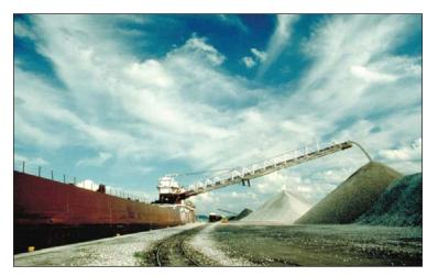
Self unloader laker vessel unloading limestone Source: U.S. Army Corps of Engineers
