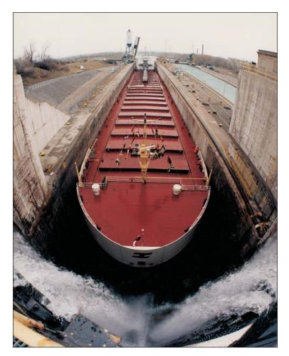
Vessel being raised in a lock Source: The St. Lawrence Seaway Management Corporation
