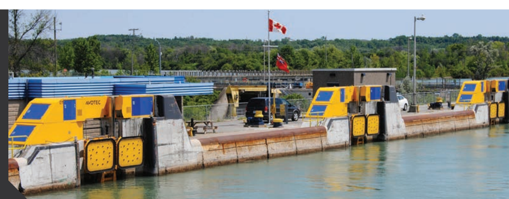
Hands Free Mooring units waiting to secure a ship
