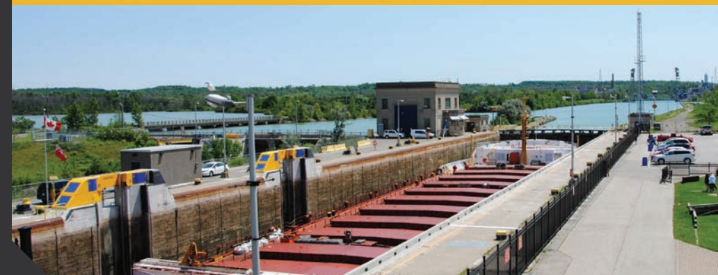
Ship secured by Hands Free Mooring (no need for wire or rope lines)
