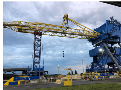
The Tug and Tow, Sara Dann and "Big Blue" crane, with the U.S. Navy's gantry crane entering Eisenhower Lock. The 170-ton crane (lifting capacity at 65') assembly, nicknamed "Big Blue", weighed 2.7 million pounds and extending 221' in height with the boom fully extended.
