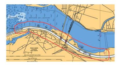
In addition, no ship shall meet another ship within the area between the caution signs that can be found on both sides of the CPR bridge (7a/7b) of the South Shore Canal.
