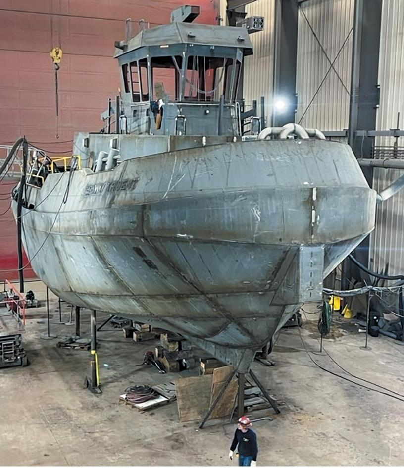
The SEAWAY TRIDENT tugboat, measuring 60 feet in length overall compared to the GUARDIAN's 118 feet, will be the companion tug to the SEAWAY GUARDIAN and will also be equipped with an ice scraping arm to help clear the lock walls of ice.
