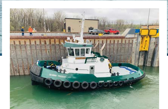
Above: The SEAWAY TRIDENT tugboat, measuring 60 feet in length overall compared to the Guardian's 118 feet, is the little sister to the SEAWAY GUARDIAN and has many of the same design characteristics. Right: The SEAWAY TRIDENT is rightsized for maneuvering inside lock chambers, with a wide 28-foot beam to improve performance in ice and enhance stability for deck crane operations.
