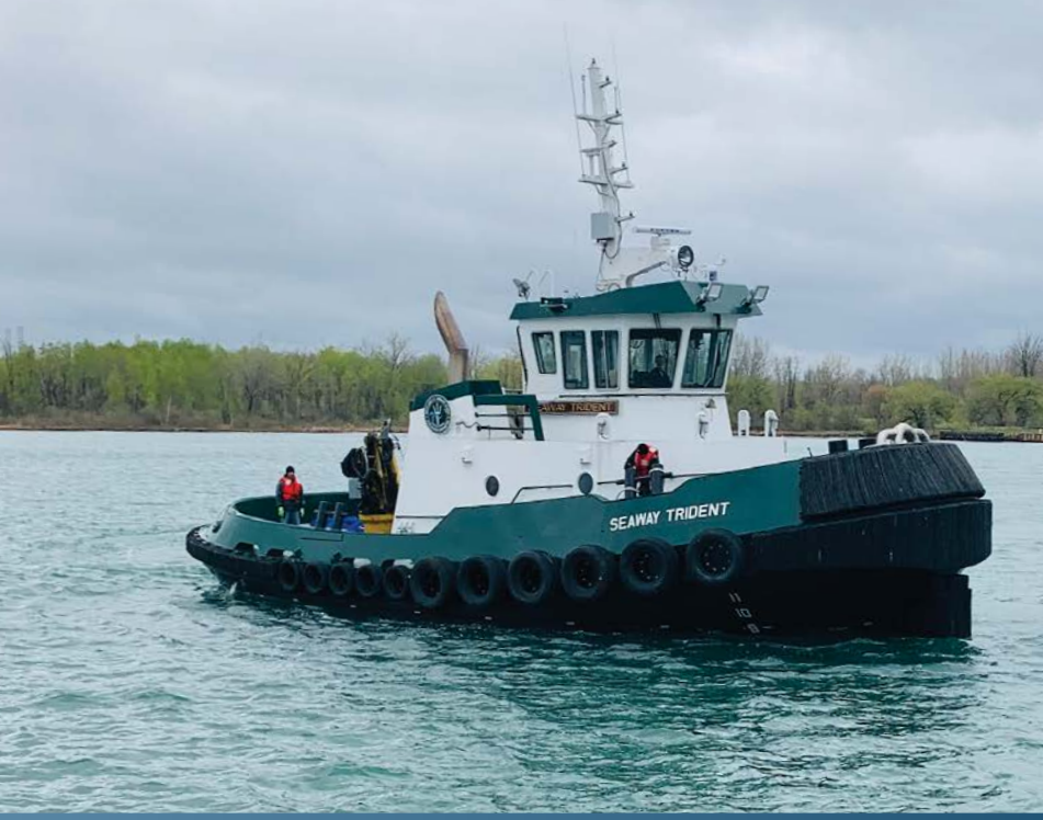
Above: The SEAWAY TRIDENT tugboat, measuring 60 feet in length overall compared to the Guardian's 118 feet, is the little sister to the SEAWAY GUARDIAN and has many of the same design characteristics. Right: The SEAWAY TRIDENT is rightsized for maneuvering inside lock chambers, with a wide 28-foot beam to improve performance in ice and enhance stability for deck crane operations.
